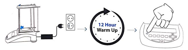
The balance must be plugged into the mains power and turned on for a minimum of 12 hours, prior to any calibration and use. The balance should then be calibrated before use.
